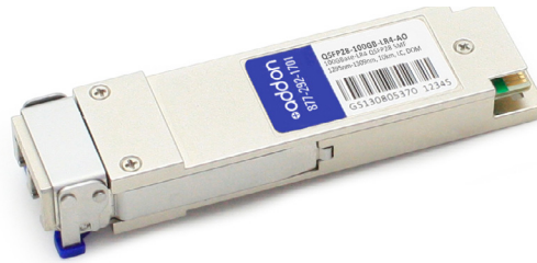
Figure 3: The QSFP28-100GB-LR4-AO is a 100 Gbps QSFP transceiver suitable for distances of up to 10 km.
