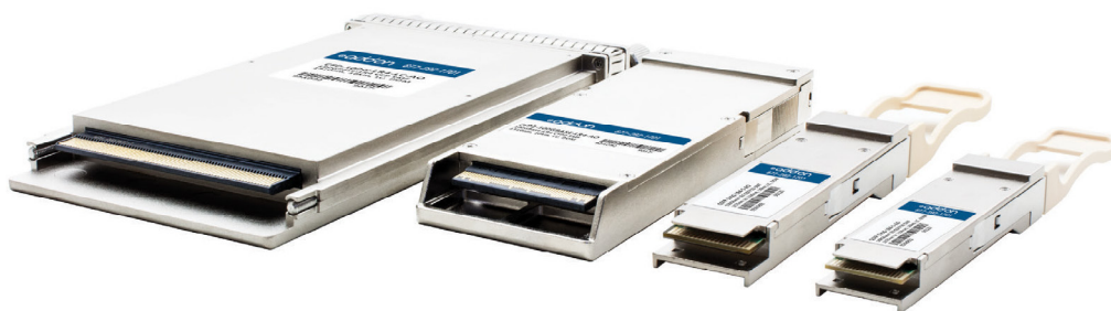
Figure 4: Network designers have a choice of transceiver form factors, including (from left) the CFP, the CFP2, the CFP4, and the QSFP28.
